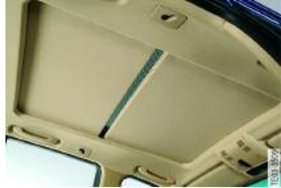
Ventilation Gap E61
